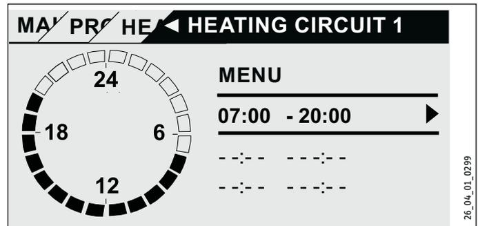
You can set three switching time pairs per day or block of days. The switching time pairs are shown on the display, to the right of the clock. Each switching time pair consists of a start time and an end time.
