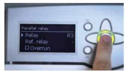
The SOM 10 features a full graphic display capable of showing historical sensor data and multiple sensors and relay values at once.
